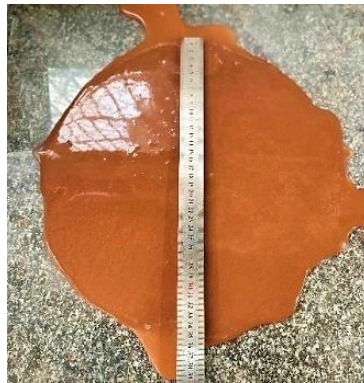
Fig. 11. Segregation observed in specimen C10W58P0.2 .
