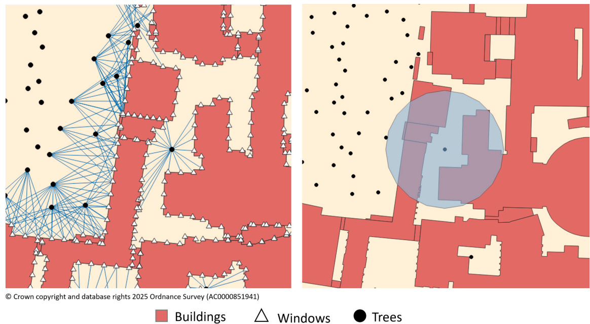
Fig. 3. Comparison of the simple and detailed methods for the 3-tree test. The detailed method (left) demonstrates lines-of-sight from ‘windows’ to trees, with the maximum length of lines-of-sight set at 30 m. The simple method (right) demonstrates a 30 m buffer around one tree, to show its overlap with the surrounding buildings. Tree data: Copyright © Bluesky International Ltd 2023. ALL RIGHTS RESERVED. ALL DATA IS PROVIDED “AS IS” AND Bluesky International Ltd EXCLUDES ALL LIABILITY HOWEVER ARISING IN RELATION TO THEM (EXCEPT FOR LIABILITY THAT BY LAW WE CANNOT EXCLUDE).
