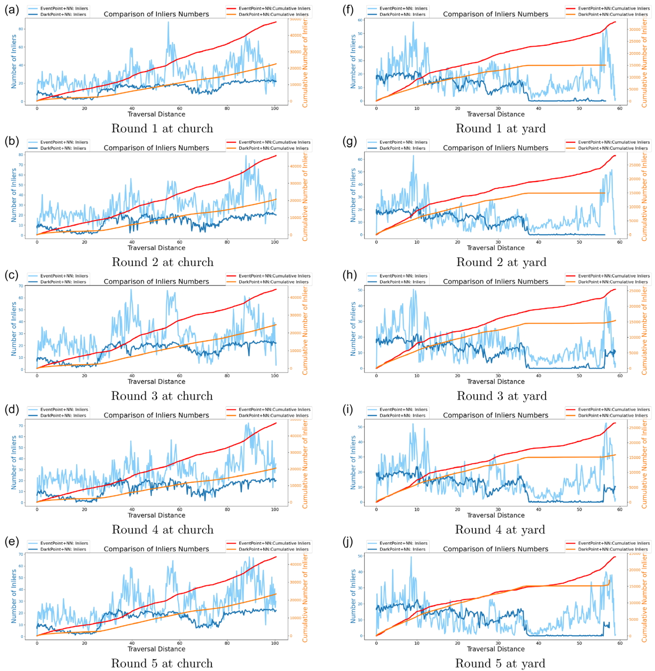
FIGURE 12 | Quantitative inlier comparisons. Left: (a)–(e) results of experiments at church between 2:00 am–3:00 am. Right: (f)–(j) results of experiments at building yard between 00:30 am–2:00 am. EventPoint achieved 113%, 124%, 76%, 134%, and 83% more accumulated inliers than DarkPoint in a, b, c, d, and e, and 147%, 80%, 68%, 69%, and 55% more in f, g, h, i, and j).
