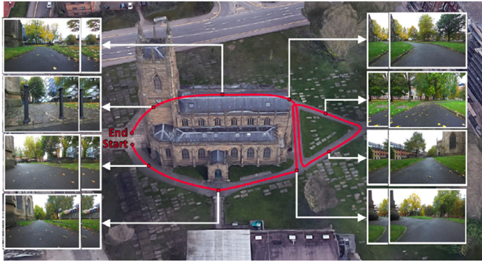
FIGURE 2 | Teleoperation in the grounds of a former church for map generation. In the teach phase a sequence of image pairs from a stereo camera are captured, some exemplar image pairs are shown superimposed on a background aerial image of the church and its surroundings.
