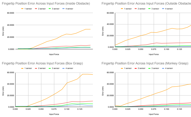
Fig. 7: Fingertip position error results across varying scenarios showing similar trends and further reaffirming the necessity for at least 2 sensors to estimate the pose when the gripper is deformed externally.
