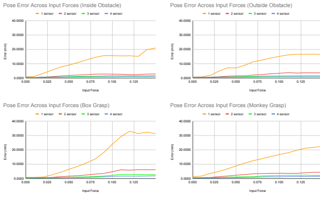
Fig. 6: Pose error results across varying scenarios showing similar trends, crucially, the necessity for at least 2 sensors to estimate the pose when the gripper is deformed externally.
