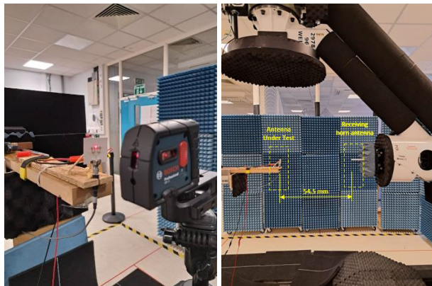
FIGURE 19. Measurement setup inside the anechoo chamber.
