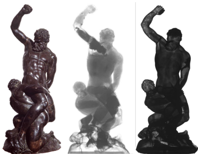
FIGURE 6 A multimodal view of the sculpture Samson Slaying a Philistine . Pictured are (left) a visual reference photograph, (centre) a neutron radiograph, and (right) an X-ray radiograph. The neutron image reveals organic fillers and restoration materials, while the X-ray image highlights dense metal, showing casting defects and internal supports. Together, they provide a comprehensive, non-invasive understanding of the object's structure and history. Reproduced from Ref. 62 under CC BY 3.0
