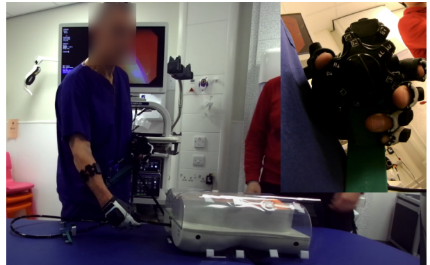
Fig. 1 Experimental setup involving a colon model with a clinician wearing data gloves and sEMG armbands.
