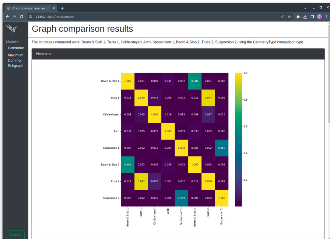
Fig. 29. An output from the PBSHM framework on computing the similarity of eight real-world bridge structures using the Jaccard Index. The bridges included within the comparison are the same set of bridges used by Gosliga et al. [20].
