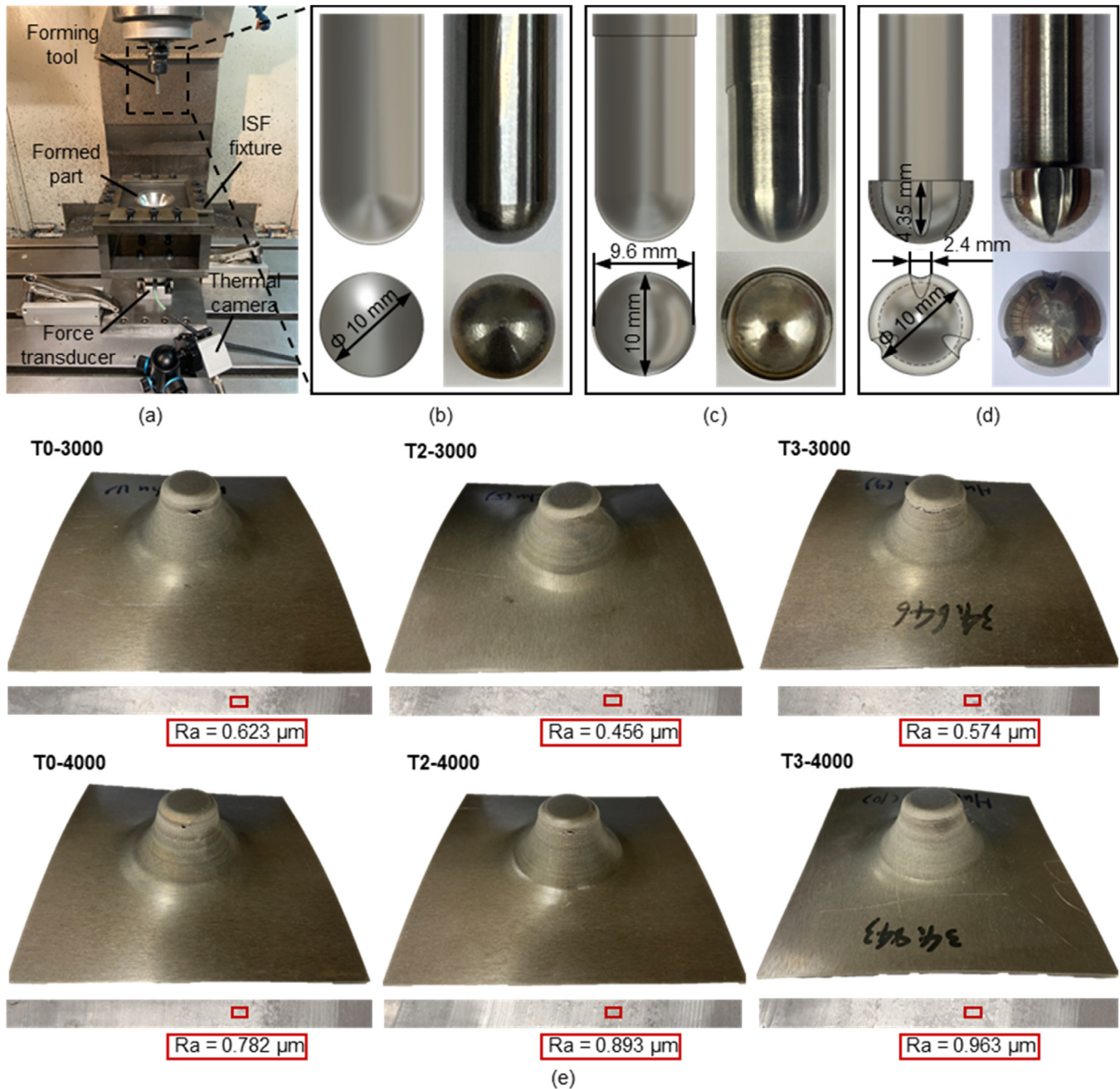
Fig. 2. Experimental setup, forming tools and formed parts of FS-ISF and RV-ISF. (a) Experimental setup including forming and measurement systems. (b) Conventional hemispherical tool T0. (c) Double-offset tool T2 with 0.2 mm offset on both sides. (d) Three-groove tool T3 with grooves on the tool surface. (e) Images of formed conic parts by FS-ISF and RV-ISF and locally scanned tool-sheet contact surface and surface roughness from the bottom of formed parts at a drawing angle of 40^\circ .
