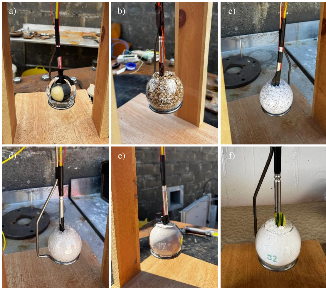
Figure 2: Examples of the mitigant materials packed inside the glass spheres, around the charge. a) water, b) vermiculite, c) perlite, d) silica gel crystals, e) fuse sand, f) Sipernat
