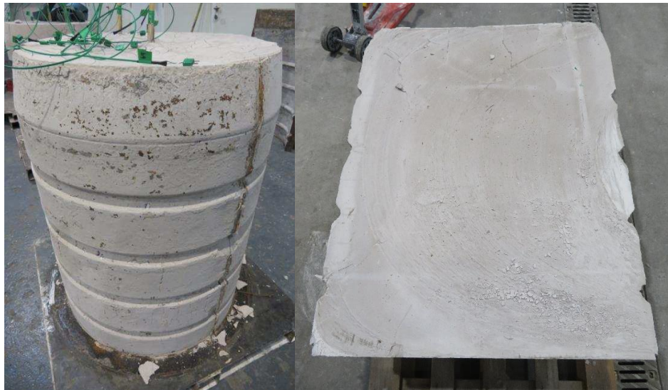
Figure 14: Demoulded 500 L product from mix 5G35 (left). Product interior surface after sectioning (right).
