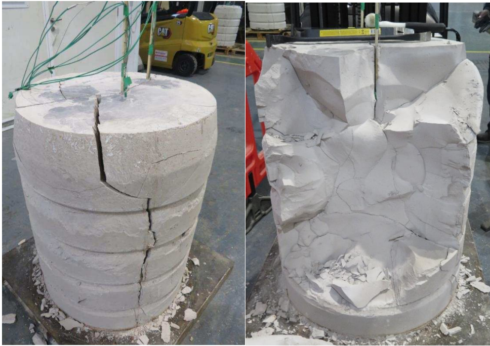
Figure 13: Demoulded 500 L product from mix 5G20 (left). Product broke up upon handling (right).
