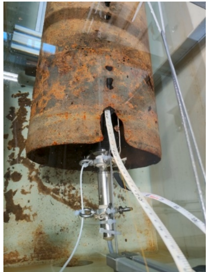
Fig. 9. A photograph of the pipe setup with the vector hydrophone inserted in the pipe at one end and speaker at the opposite end.
