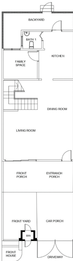
Figure 7. H2_JP_MLY repurposed the entrance porch as a buffer between the private outdoor and indoor areas and extended the TV room, tactically separating the front house for temporary hosting guests while the rear of the house for privacy and modesty. (source: Authors).
