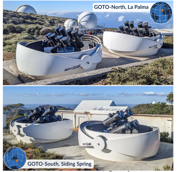
Figure 1. The full configuration of the GOTO telescope network in April 2023, comprising 32 robotic unit telescopes distributed across four domes, two domes at each of the two sites. Top: GOTO-N, located at the Observatorio del Roque de los Muchachos on La Palma, comprising GOTO-1 (left) and GOTO-2 (right). Bottom: GOTO-S, hosted at Siding Spring Observatory in Australia, consisting of GOTO-3 (left) and GOTO-4 (right). Figure credit: Dyer et al. 2024 .
