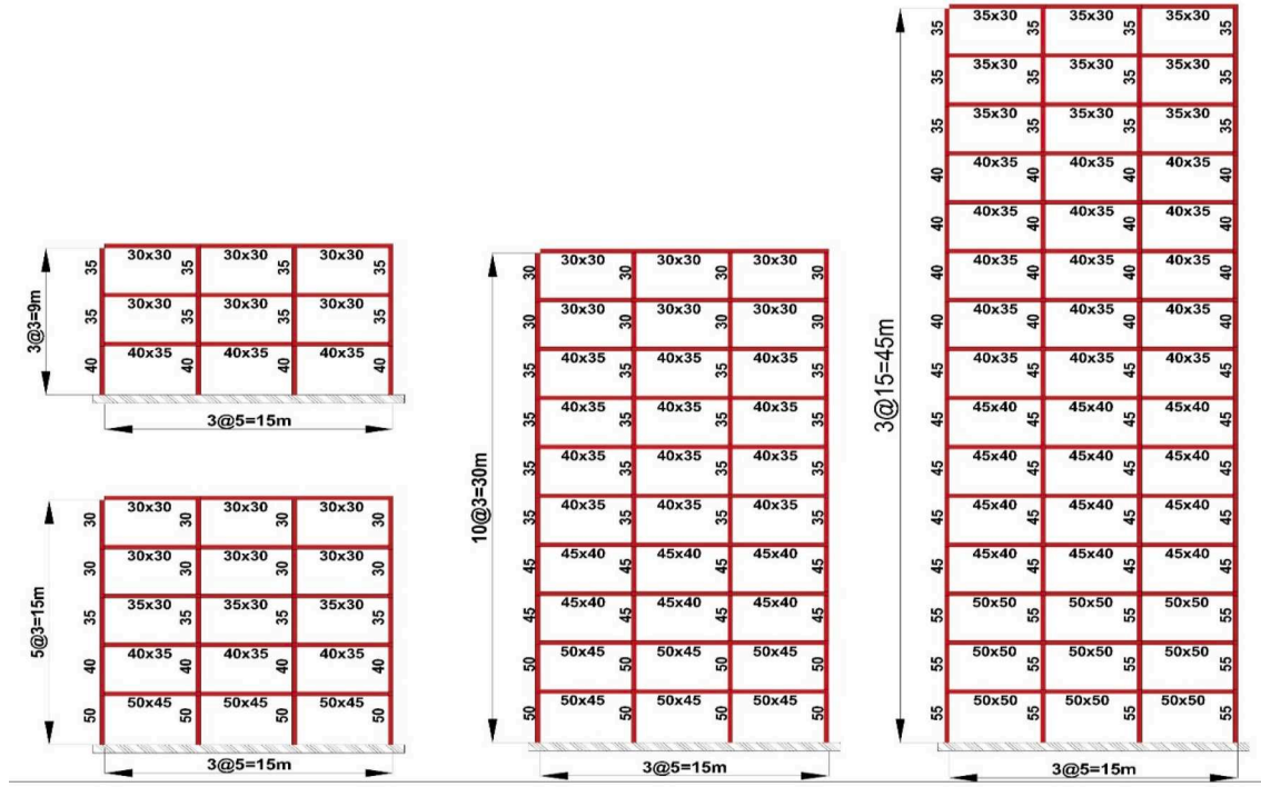
Fig. 1. Geometry and dimensions of beam and column members of 3-, 5-, 10- and 15-storey RC frames (Beams: “height × width”; Columns: “square dimension”).
