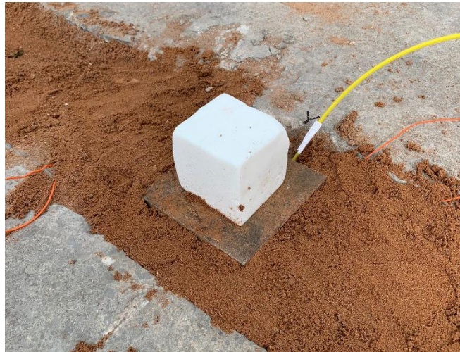
Figure 1: Anvil mounted 1:1:1 PE4 cube charge
