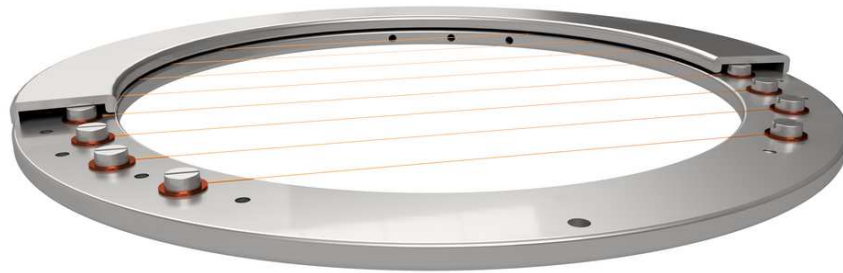
Figure 2. CAD image of the anode electrode. The gold-plated tungsten wires of 10 \mu\text{m} diameter are fixed to the stainless steel support frame by means of copper washers and stainless steel bolts. To increase visibility, the wire diameter is enlarged in the image. By using every second wire position, a 10 mm wire pitch is achieved. Only half of the stainless steel piece to cover the screws is shown.
