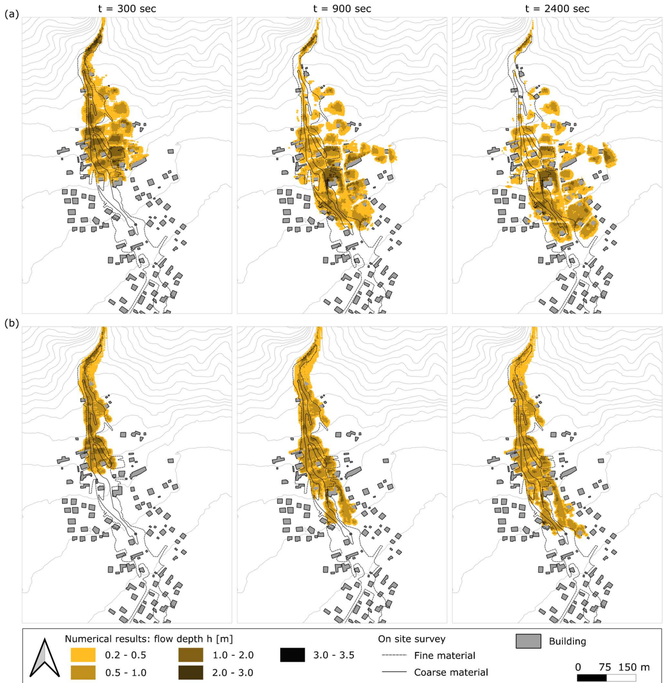
Fig. 12 Simulated runoff after the simplified triggering approach and comparison with surveyed flooded area: results using a a Voellmy rheology with \tan \delta = 0.1 and \xi = 500 \text{ m/s}^2 , and b a Bingham rheology with \tau_0 = 1300 \text{ Pa} and \mu_B = 80 \text{ Pa}\cdot\text{s}
