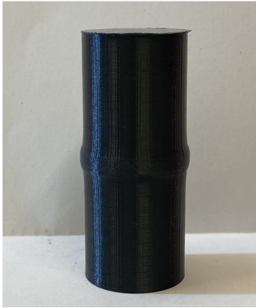
Figure 10. Inelastic deformation mechanism due to pore space collapse in FDM printed sample with a large oblate pore (1.4).
