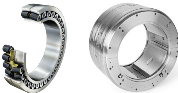
Figure 3. The left-hand panel shows a Schaeffler roller bearing for the main shaft of a wind turbine [27] while the right-hand panel shows an example of a Miba tilting pad journal bearing used in turbines [28]. In both examples sensors could be placed on the outside of the casing before putting the bearing in its mounting.
