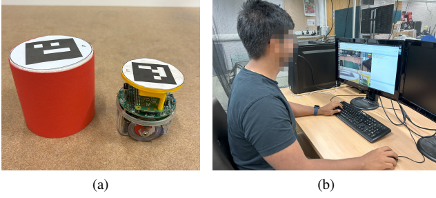
Fig. 3. Tasks and actors: (a) Red cylindrical objects, used to represent tasks, and Pi-puck robots. Each object and Pi-puck have an ArUco marker that is detected by the overhead camera. (b) Each operator interacts with the user interface and guides one of the robots representing lead agents.
