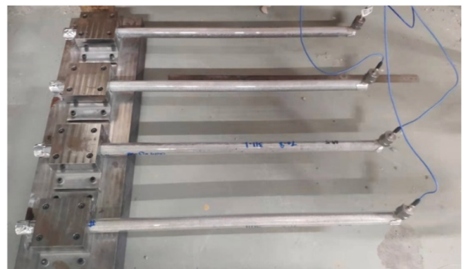
Fig. 3. Equipment for elastic modulus measurement.
