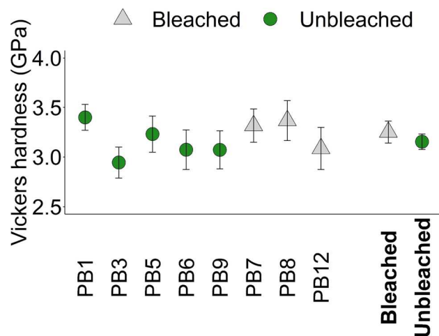
Fig. 5 Mean Vickers hardness of five unbleached and three bleached coral skeletons, with error bars representing 95% confidence intervals calculated across 21–33 coral scars per sample (total n=210 ). The mean Vickers hardness for pooled bleached (B) and unbleached (UB) corals is additionally shown in bold
