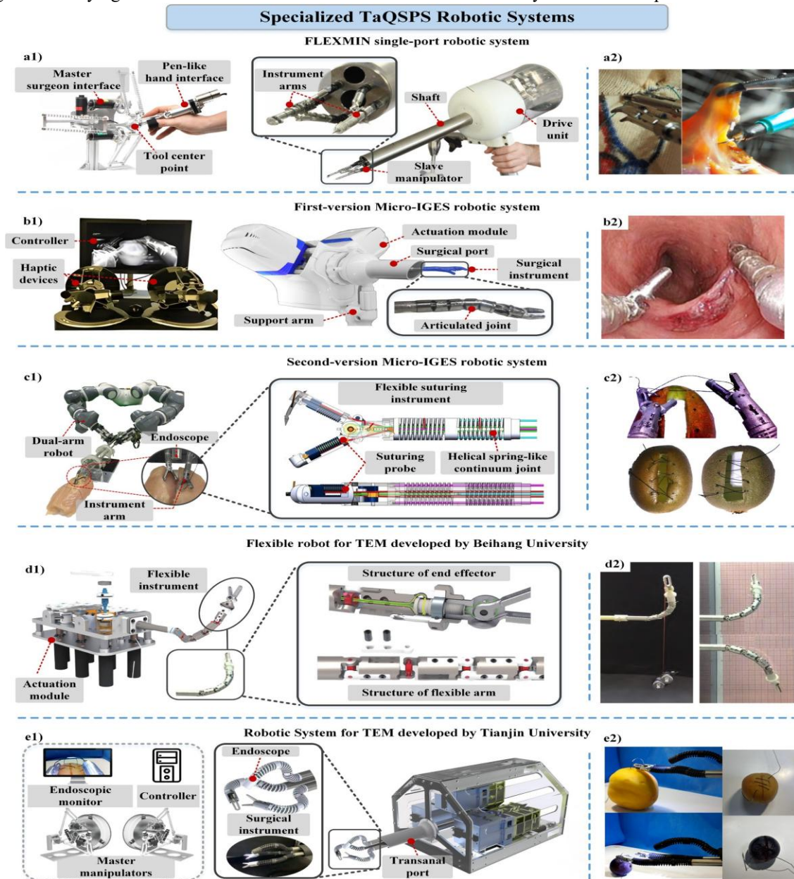
Fig. 5. Specialized taQSPS robotic systems: a1) The master surgeon interface and slave robot of FLEXMIN single-port robotic system [66], [67], © 2015 IEEE and © 2017 IEEE; a2) Experimental testing of FLEXMIN using a porcine model [67], © 2017 IEEE; b1) The master console and slave manipulator of First-version Micro-IGES robotic system [68], [69], © 2017 IEEE; b2) In-vivo tests of first-version Micro-IGES robotic system [69], © 2017 IEEE; c1) The dual-arm robot and suturing instruments of Second-version Micro-IGES robotic system [70], © 2019 IEEE; c2) Suturing and knot-tying experiments of secondversion Micro-IGES robotic system [70], © 2019 IEEE; d1) Flexible robot for TEM developed by Beihang University and its joint structure [72], © 2023 ROBOT; d2) Motion performance experiments of flexible robot for TEM developed by Beihang University [72], © 2023 ROBOT; e1) Master control components and slave manipulator of Robotic System for TEM Developed by Tianjin University [73], © 2024 IEEE; e2) Surgical simulation experiments of robotic System for TEM Developed by Tianjin University [73], © 2024 IEEE.
