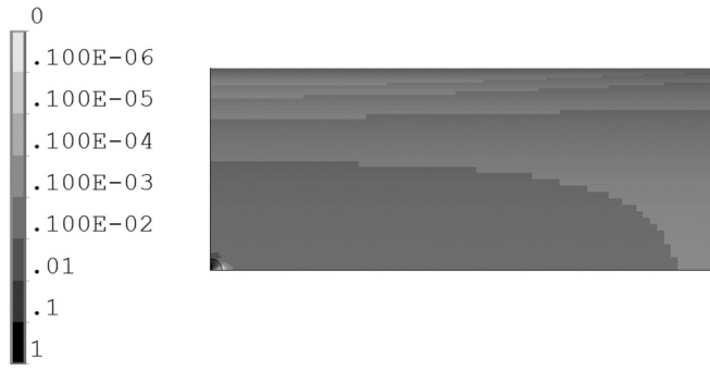
Fig. 12. FEA predicted Effective Volume weighting, (\sigma_{a,SWT}/\sigma_{a,SWT,max})^{M_{ES}} , for the sharp notch bending specimen under bending loading for the quarter-pipe model showing the weighting assigned to elements away from the notch. The axial direction is left-to-right, and the notch is located at the bottom left.
