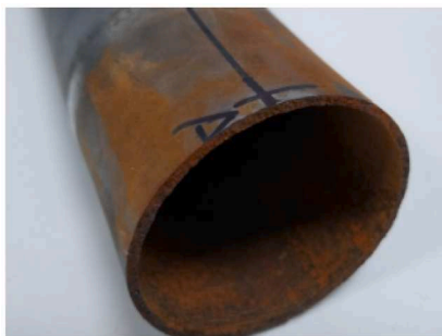
Fig. 3. Examples of fractured specimens post-test including (a-b) uniaxial specimens still secured in the fatigue test machine, and (c-d) the circumferential fractures observed at the midpoint of specimens subjected to bending fatigue loads.
