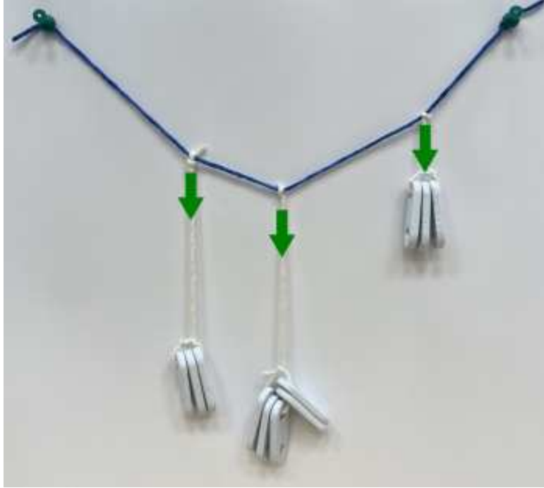
Figure 1: A funicular polygon generated by hanging loads on a cable or thread (in blue), the weight of which is negligible.
