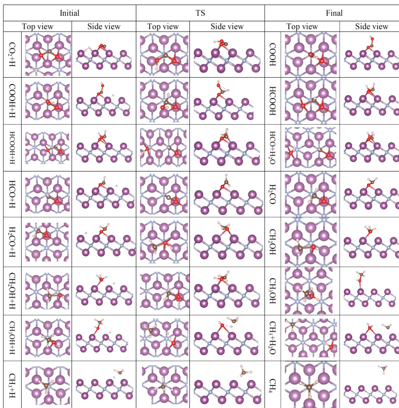
Figure 12. The selected reactions with their corresponding initial, transition (TS) and final states at the \text{Sc}_2\text{N}(001) surface (Sc = purple, N = blue, O = red, C = brown, H = white).
