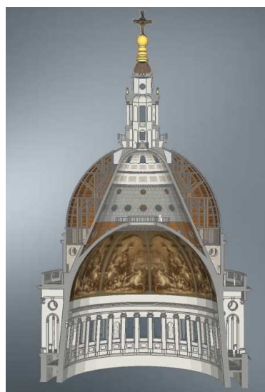
Figure 1. Cross section of the three parts of the dome: interior dome of brick; middle-inner cone of brick; wooden outer dome covered in lead on the exterior. This was created in a 3D virtual model from [5], reproduced with permission.
