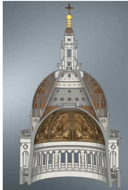
Figure 1. Cross section of the three parts of the dome: interior dome of brick; middle-inner cone of brick; wooden outer dome covered in lead on the exterior; as created in a 3D virtual model from [5], reproduced with permission.
