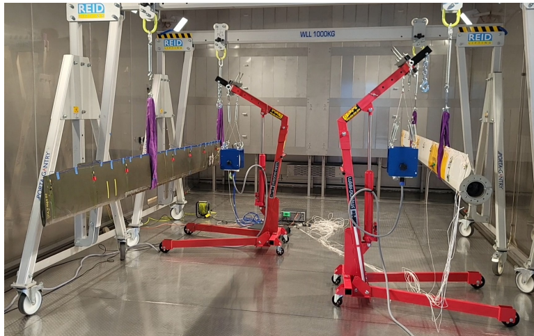
Figure 6: The experimental setup to perform modal testing on a metal (right) and composite (left) blade simultaneously.
