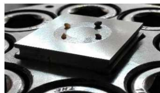
(b) sand manually placed on the bottom HPT sample
