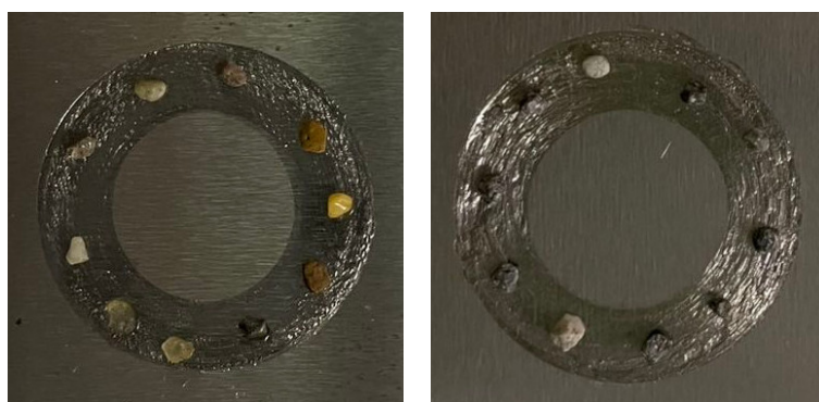
(a) Sand placement on bottom HPT sample, left GB sand, right AT.
