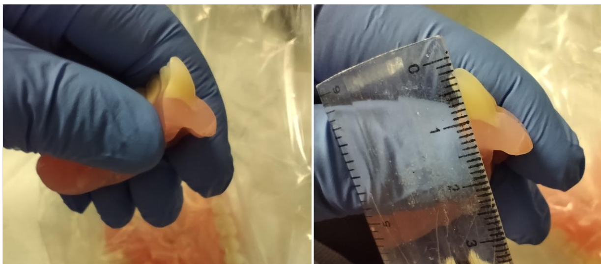
Figure 2: Photos of a fractured 3D printed denture. Note the shear fracture, likely an artifact of the material properties of the denture, despite the acrylic base material thickness measuring 5mm at the point of fracture.
