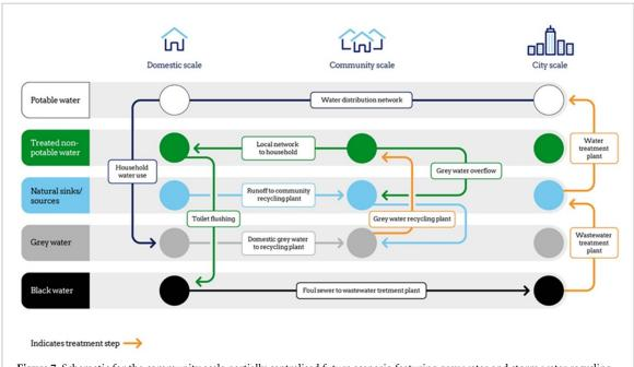
**Figure 7.** Schematic for the community scale partially centralised future scenario featuring grey water and storm water recycling at local scale. Reproduced with permission from Twenty65, <a href="https://www.twenty65.ac.uk">www.twenty65.ac.uk</a>.
