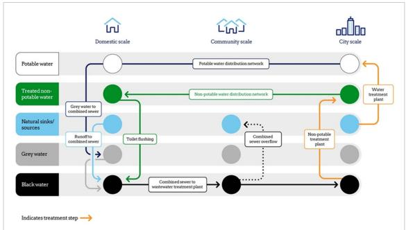
**Figure 6.** Schematic for the dual distribution future scenario featuring non-potable water distribution at city scale. Reproduced with permission from Twenty65, <a href="https://www.twenty65.ac.uk">www.twenty65.ac.uk</a>.
