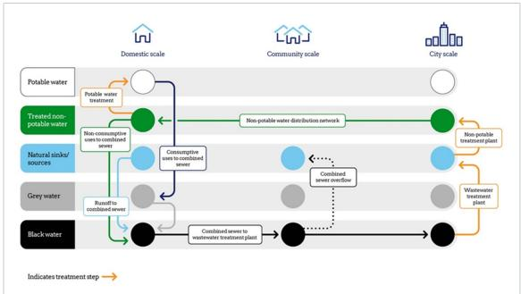
**Figure 5.** Schematic of point of use treatment scenario featuring city-scale distribution of non-potable water with domestic treatment at household scale. Reproduced with permission from Twenty65, <a href="https://www.twenty65.ac.uk">www.twenty65.ac.uk</a>.
