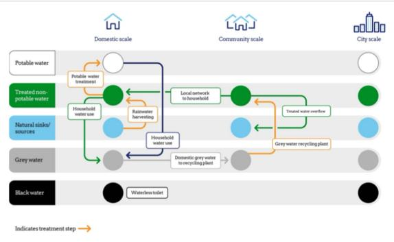
**Figure 8.** Schematic for the fully decentralised future scenario featuring domestic scale treatment supplemented by community scale pooled water resources and waterless toilets. Reproduced with permission from Twenty65, <a href="https://www.twenty65.ac.uk">www.twenty65.ac.uk</a>.
