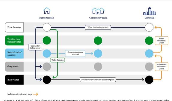
**Figure 4.** Schematic of 3 by 5 framework for infrastructure scale and water quality, mapping centralised water and sewer networks and treatment. Reproduced with permission from Twenty65, <a href="https://www.twenty65.ac.uk">www.twenty65.ac.uk</a>. Adapted from Hook *et al* 2018.
