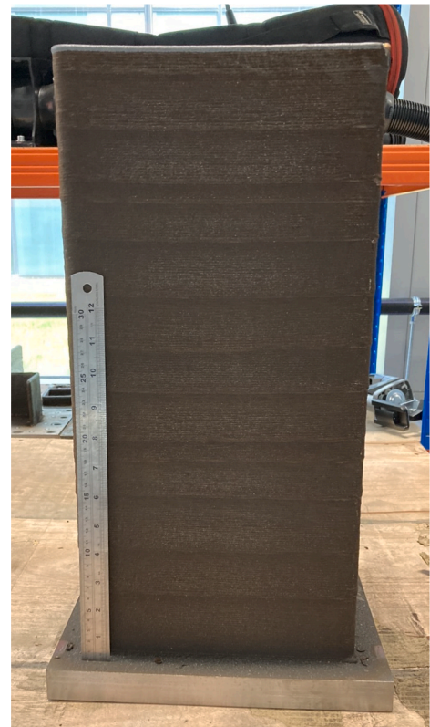
Fig. 2. The process of producing WAAM specimens: (a) parent material design, (b) extraction plan, (c) additive manufacturing via robotic cell, and (d) final parent material product.
