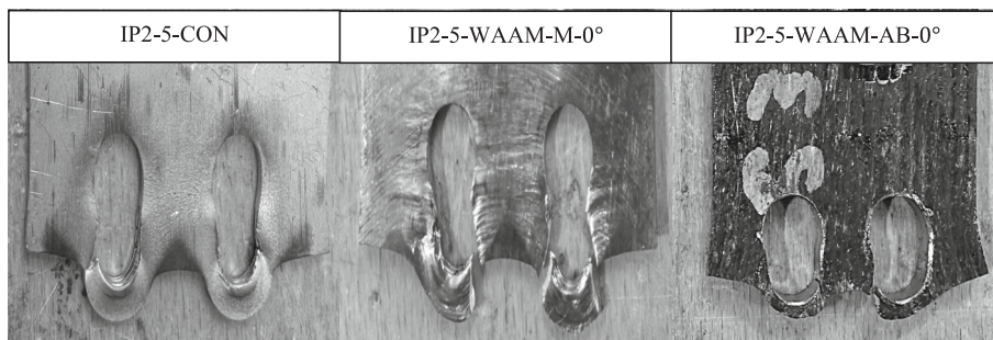
Fig. 18. Failure modes for IP2-5 configuration of CON and AM plates.
