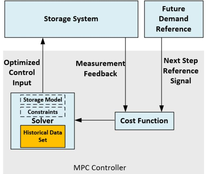
Fig. 3. Historical Data Handling in MPC Based Energy Storage Management
