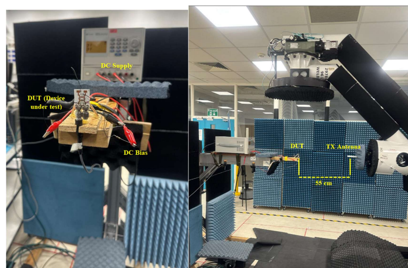
Figure 12. Radiation pattern measurement setup.
