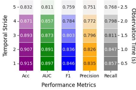
Fig. 6. Performance of PIP-Net- \alpha across different temporal resolutions: As the stride increases, the sampling frequency decreases, expanding the observation time from 0.5 to 2.5 seconds, influencing the model’s ability to predict pedestrian crossings.
