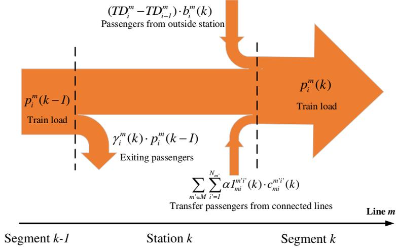
Figure 1: Illustration of passenger load dynamic of train  $i$  at station  $k$ .
