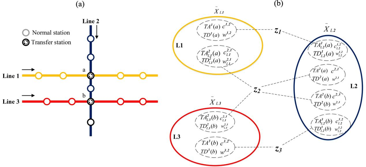
Figure 3: (a) Map of a three-line metro network; (b) Illustration for the decomposition and consensus optimization.
