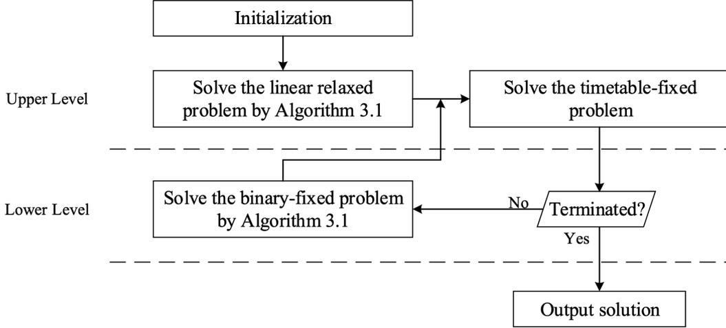
Figure 5: The flowchart of Algorithm 3.2.
