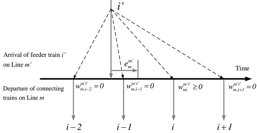
Figure 2: Illustration of transfer waiting time.
