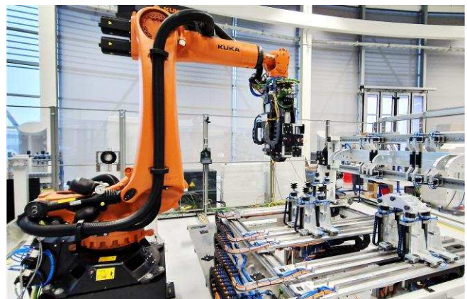
Figure 1: The robotic drilling cell with reconfigurable fixturing.
