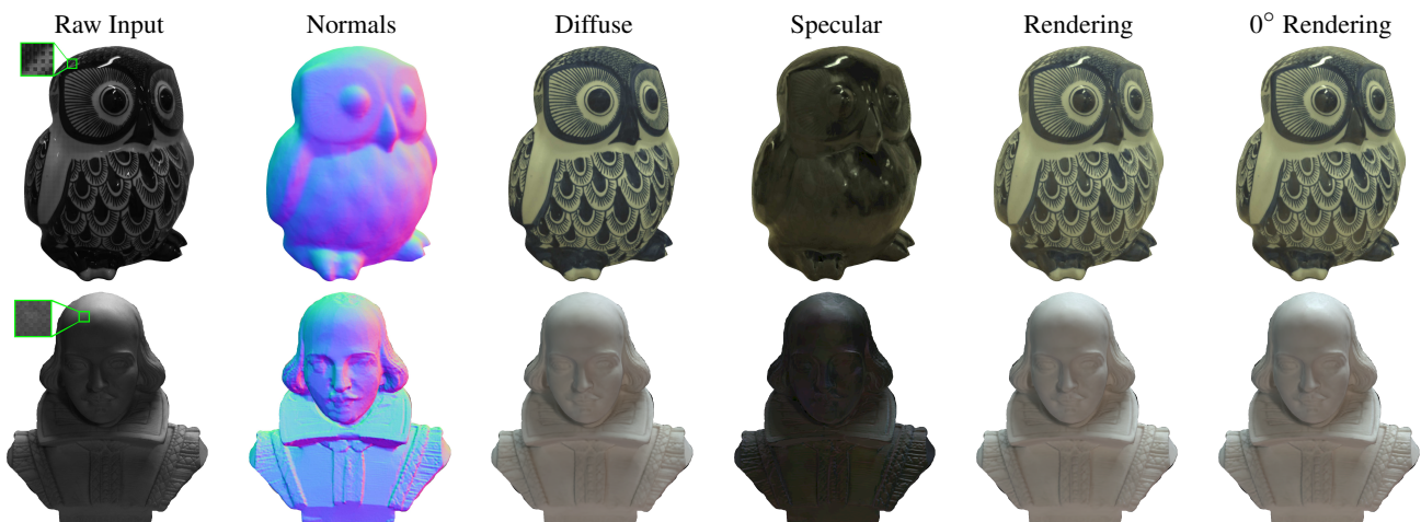
Figure 1: From multi-view raw division-of-focal-plane colour-polarisation images (one input view in Col. 1), we reconstruct a neural SDF (surface normals, Col. 2) and neural fields for diffuse and specular radiance (Cols. 3–4). Col. 1 includes a zoom-in inset that enlarges a 16 \times 16 patch of the Colour Polarisation Filter Array (CPFA), revealing its mosaic pattern. Combining the two radiance fields yields unpolarised radiance (Col. 5). From this representation we can render colour, polarised images from any view; the RGB image rendered at a 0^\circ polariser angle appears in Col. 6. All images are rescaled and tone-mapped for display.
