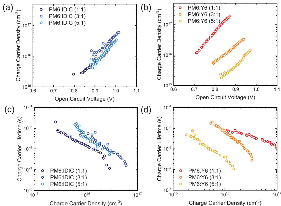
**Figure 6.** Charge carrier density and lifetime study in devices at open circuit voltage. Charge extraction data as a function of light intensity allow determination of charge density versus open circuit voltage, as plotted for a) PM6:IDIC and b) PM6:Y6 solar cells for different D:A ratios. Charge carrier lifetime versus charge carrier density determined from charge extraction and transient photovoltage measurements for different donor-acceptor ratios for c) PM6:IDIC and d) PM6:Y6 solar cells.
