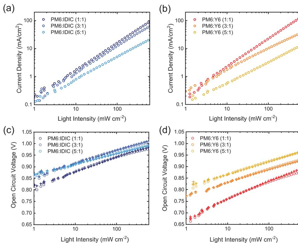
**Figure 5.** Intensity-dependent device analysis. Light intensity-dependent short circuit current of a) PM6:IDIC and b) PM6:Y6 solar cells with various D:A ratios. Light intensity-dependent open circuit voltage measured (circle) and reconstructed (cross)<sup>[47]</sup> of c) PM6:IDIC and d) PM6:Y6 solar cells with various D:A ratios blend.
