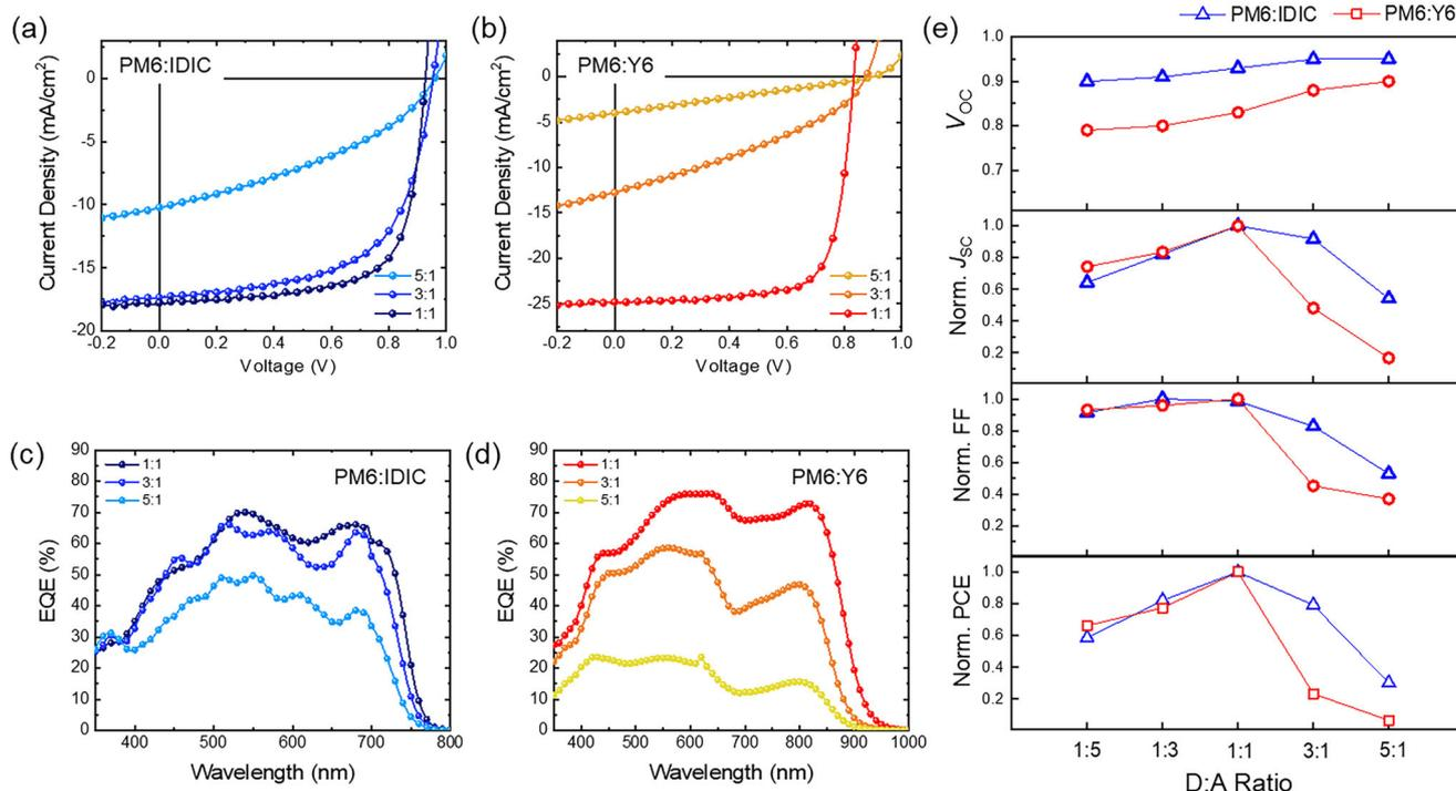
**Figure 1.** Device performance and electrical parameters comparison.  $J$ - $V$  characteristics of a) PM6:IDIC and b) PM6:Y6 solar cells. EQE spectra of c) PM6:IDIC and d) PM6:Y6 solar cells. e) Comparison of device parameters ( $V_{OC}$ ,  $J_{SC}$ , FF, and PCE) for PM6:IDIC and PM6:Y6 solar cell devices.
