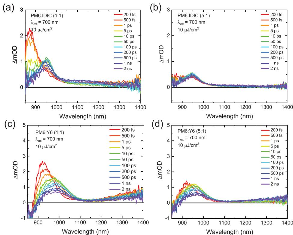
**Figure 3.** Ultrafast transient absorption study. Transient absorption spectra with respect to wavelength as a function of time delay for PM6:IDIC blends with a) 1:1 and b) 5:1 ratio and PM6:Y6 blends with c) 1:1 and d) 5:1 ratio excited at 700 nm,  $10 \mu\text{J cm}^{-2}$ .
