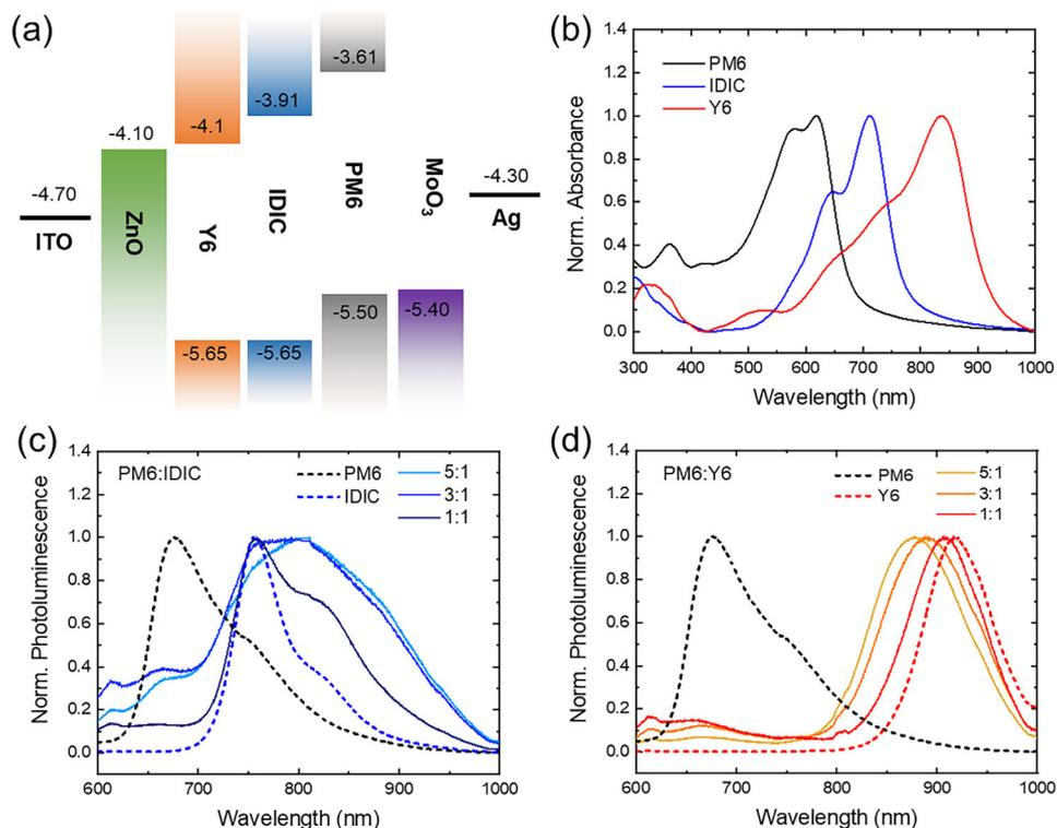
**Figure 2.** The energy level and study state optical analysis. a) Approximate electronic energy levels of the materials used in this work in thin films, obtained from the literature measured by cyclic voltammetry;<sup>[37–39]</sup> b) Normalized UV-vis absorption spectra for neat material films. Normalized PL spectra with 532 nm excitation wavelength of c) PM6:IDIC and d) PM6:Y6 films with varying D:A ratio, including neat materials.
