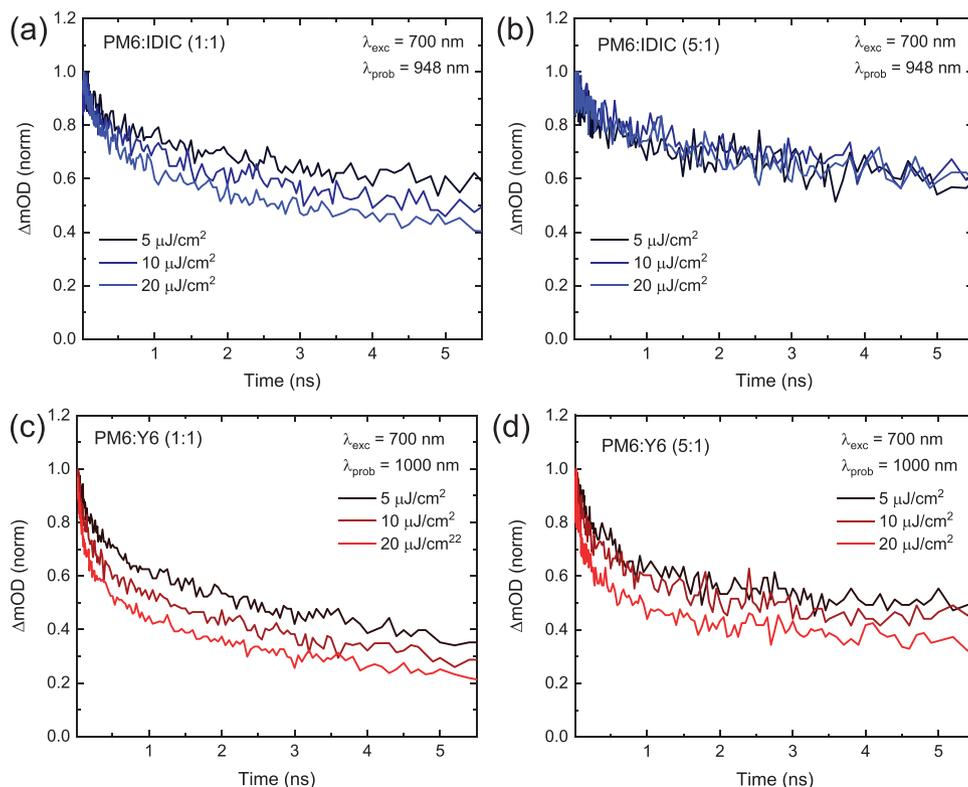
**Figure 4.** Kinetic response of ultrafast transient study. Pump fluence-dependent transient absorption traces of PM6:IDIC blends with a) 1:1 and b) 5:1 ratios excited at 700 nm, probed at 948 nm, and PM6:Y6 blends with c) 1:1 and d) 5:1 ratios excited at 700 nm, probed at 1000 nm. For both blend systems, the probe wavelengths correspond to CT/charge pair photoinduced absorption.
