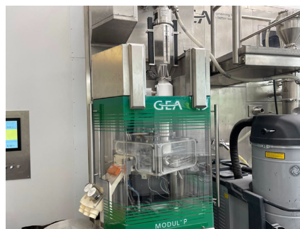
(b) The continuous rotary tablet press (GEA Pharma Systems, Collette™, Wommelgem, Belgium)
