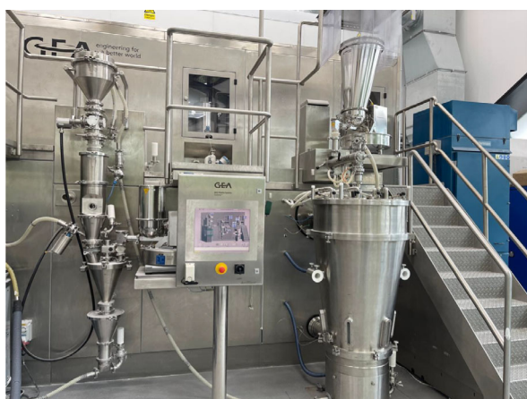
(a) The continuous powder processing line (GEA Pharma Systems, Collette™, Wommelgem, Belgium)
