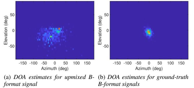
Figure 3: Directional grid of DOA estimates resulting from the time-sampled intensity vectors of the (a) upmixed B-format signals and (b) ground truth B-format signals for a source spatialised to  $\theta = \phi = 0^\circ$ .
