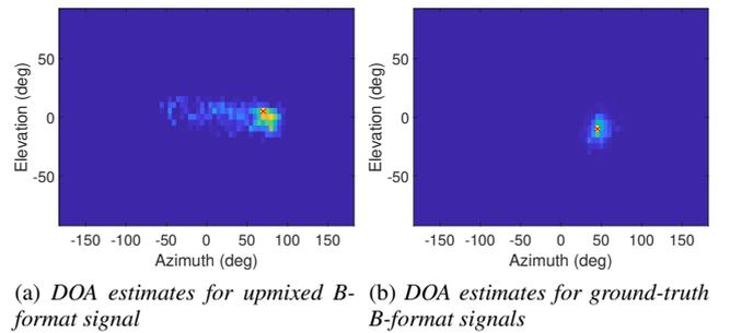
Figure 4: Directional grid of DOA estimates resulting from the time-sampled intensity vectors of the (a) upmixed B-format signals and (b) ground truth B-format signals for a source spatialised to  $\theta = 45^\circ$ ,  $\phi = 0^\circ$ .
