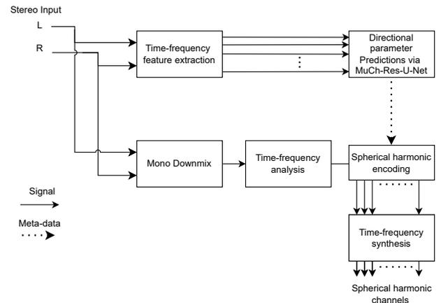
Figure 2: Block diagram of proposed stereo to B-format upmixer utilising directional parameters predicted by MuCh-Res-U-Net
