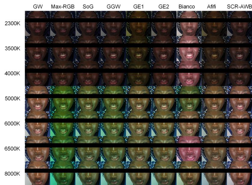
**Figure 7.** Comparison of different AWB algorithms of dark skin tone. Only the AWB Gain parameter is changed. The image is processed by BLC, AWB, Demosaic, CCM, and  $\gamma$  correction.
