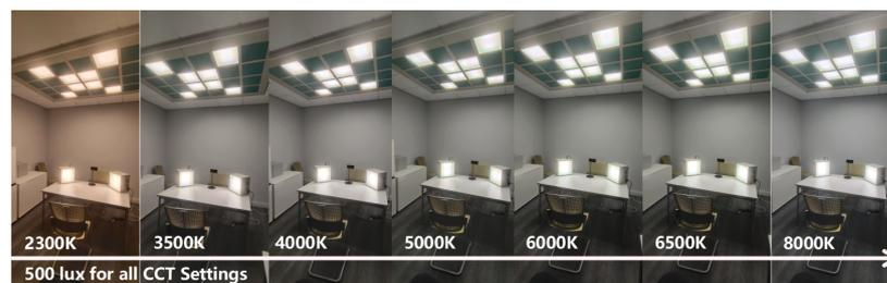
**Figure 3.** The laboratory light environment settings for Experiments 1 and 2: Experiment 1 only uses color card data shot at 2300 K, 3500 K, 4000 K, 5000 K, and 6500 K. In Experiment 2, the subjects will be shot in a total of seven different CCT scenes, and the illumination of the shooting position in the scene is set to 500 lux.
