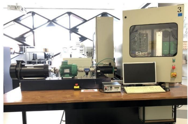
Fig. 1: Existing industrial-scale PEMD training system.
