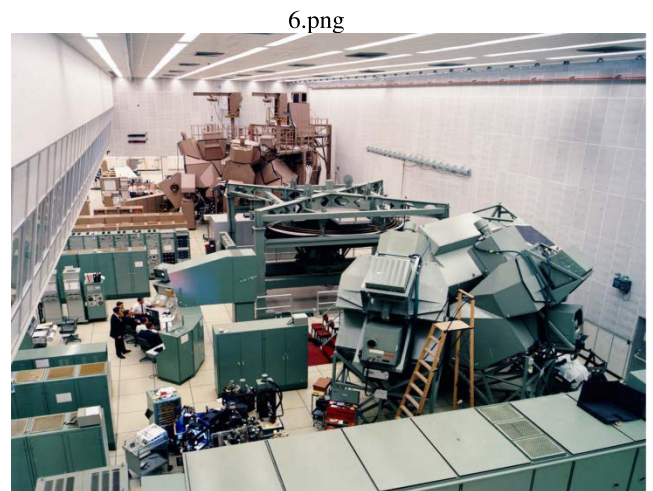
FIGURE 5. The physical twin of Apollo 13, the green side is the foreground simulator, and the brown side is the Command Module Simulator [2].
