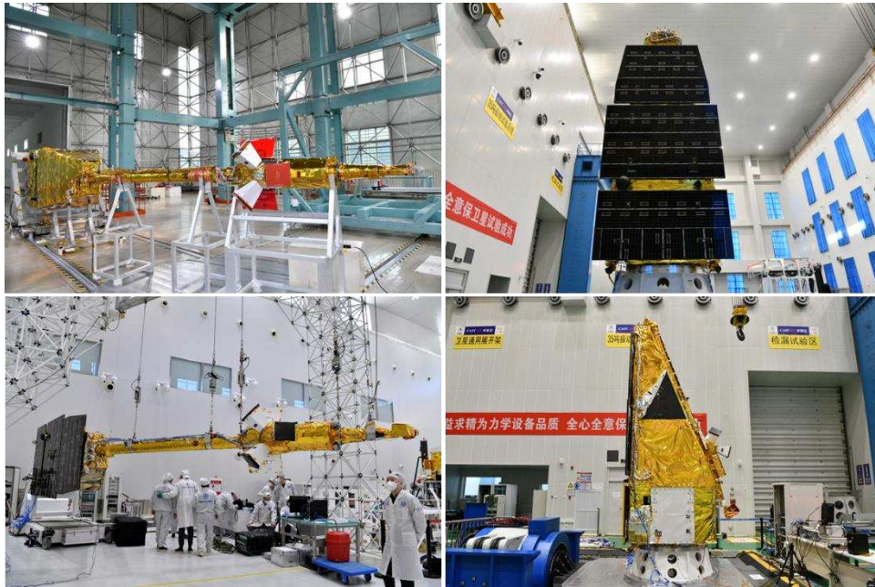
Figure 2: MSS-1A under construction (Zhang presentation). The satellite is 9m long with the boom deployed and has a mass of 570kg, carrying a payload of seven instruments.
