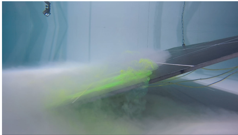
Video 2: Annotated real-time video illustrating the temporal evolution of the flow with a 20° slope. Fluorescent dye injected at a series of lateral points onto the slope surface was used to visualize the interaction of the density current and the containing topography. Gridded white lines were marked on the slope surface to aid the identification of the height at which the stable flow front developed and the maximum run-up height ( h_{\max} ).
