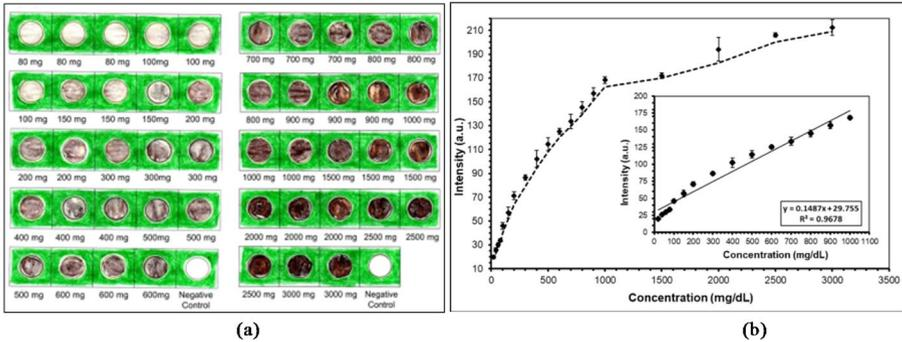
**Fig. 4** Quantification of starch adulterated milk using iodine reagent, (a) spot test images of milk spiked with starch carried on  $\mu$ -PAD spot arrays ( $5 \times 5$ ), and (b) calibration curve prepared from spot tests of milk adulterated with starch. Each data point is the average of 3 color intensities for an adulterant concentration and the error bars indicate the standard deviations
