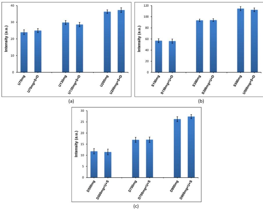
**Fig. 6** Evaluation of M- $\mu$ PAD specificity for milk samples spiked with (a) urea, (b) starch, and (c) detergent at three concentrations, and then with the other two adulterants at fixed concentrations
