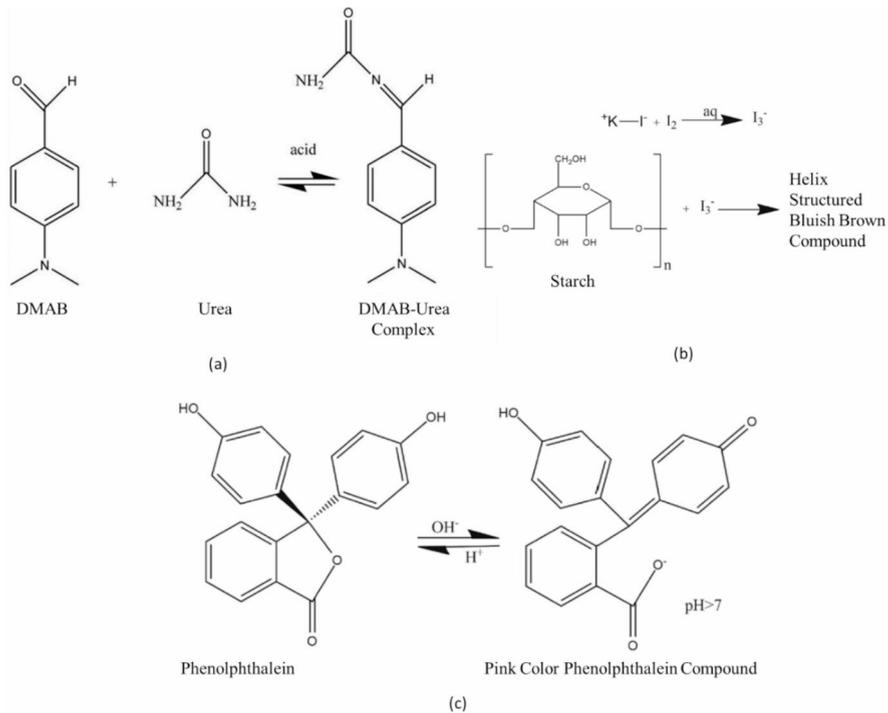
**Fig. 2** Schematic illustration of colorimetric reactions of different adulterants with corresponding reagents, (a) urea with DMAB [46], (b) starch with iodine [47], and (c) detergent with phenolphthalein [48]
