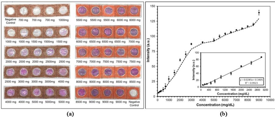
**Fig. 5** Quantification of detergent adulterated milk using phenolphthalein reagent, (a) spot test images of milk spiked with detergent carried on  $\mu$ -PAD spot arrays ( $5 \times 5$ ), and (b) calibration curve prepared from spot tests of milk adulterated with detergent. Each data point is the average of 3 color intensities for an adulterant concentration and the error bars indicate the standard deviations
