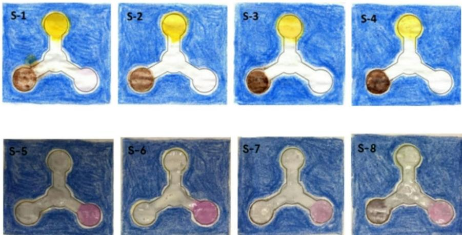
**Fig. 7** Images showing simultaneous colorimetric assays conducted on M- $\mu$ PADs for urea, starch, and detergent in eight blind milk samples with concentrations shown in Table 2
