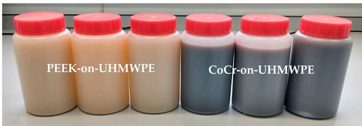
**Figure 6.** Lubricant samples from the PEEK-on-UHMWPE knee (left) and the CoCr-on-UHMWPE knee replacement (right) following 0.3 MC of wear simulation with PMMA cement particles added to the lubricant. Note the discolouration of the lubricant in the CoCr-on-UHMWPE test.
